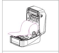
2. Load print media into the printer; adjust the paper guide to be same width of print media.
