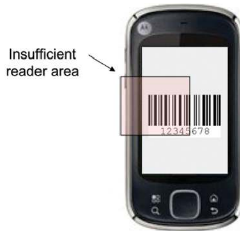
Figure 5 - Insufficient field of view
